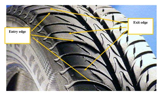
A factor with an impact on the phenomenon of "sow teeth" usage is the tread pattern. The more "open" the pattern (the farther apart the lugs of the tread from each other) the greater the risk of sow teeth usage in the tread. In terms of resistance to "sow teeth" usage, the ideal tire would be one in which the tread pattern is uniform with no voids or lugs. However, it must be remembered
